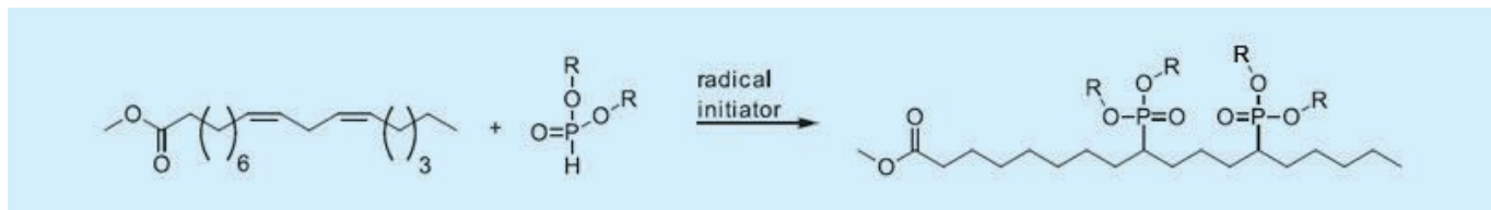
Figure 3. Dialkyl phosphonates (r=alkyl) are synthesized by using a hydrophosphonation reaction that utilized methyl linoleate. Figure courtesy of USDA.
