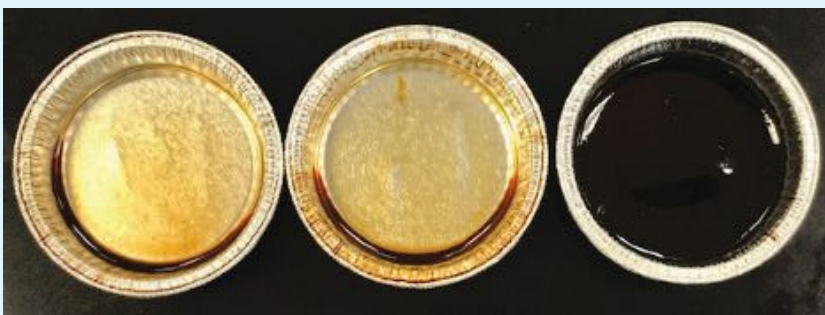
Figure 1. The improved performance of biodegradable lubricants can be shown in test results for three ISO 46 lubricants evaluated for use as chain oils. Thermal stability testing shows that the biodegradable, food-grade lubricant (middle column) displays comparable performance to an incumbent food-grade lubricant (left column) and a non-biodegradable, petroleum-based industry standard (right column). Figure courtesy of Zschimmer & Schwarz.
